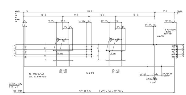
SteelCad can automatically place stiffeners at cantilevered conditions, either on the column center line as shown here, or in line with the column flanges, or you can specify a distance between stiffeners. Also, SteelCad automatically shows a section view when required, as seen with the stiffened cantilever condition shown here.
