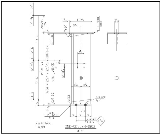
The above column was detailed in **less than a minute** using SteelCad because all the data needed to generate the detail was passed to the column from previously detailed pieces like the one on the previous page. We simply told the program on which level the beam was framing and its piece mark, and **the program did the rest!**
